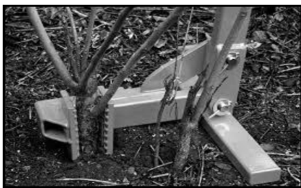
Weed Wrench's jaws clutching shrub
